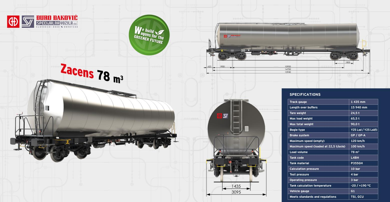
Zacens 78 m<sup>3</sup> is a specialized type of cargo wagon designed for transporting temperaturesensitive liquids, such as certain chemicals, oils, and petroleum products. The presence of a heating system makes them particularly suitable for substances that solidify or become highly viscous at lower temperatures.
