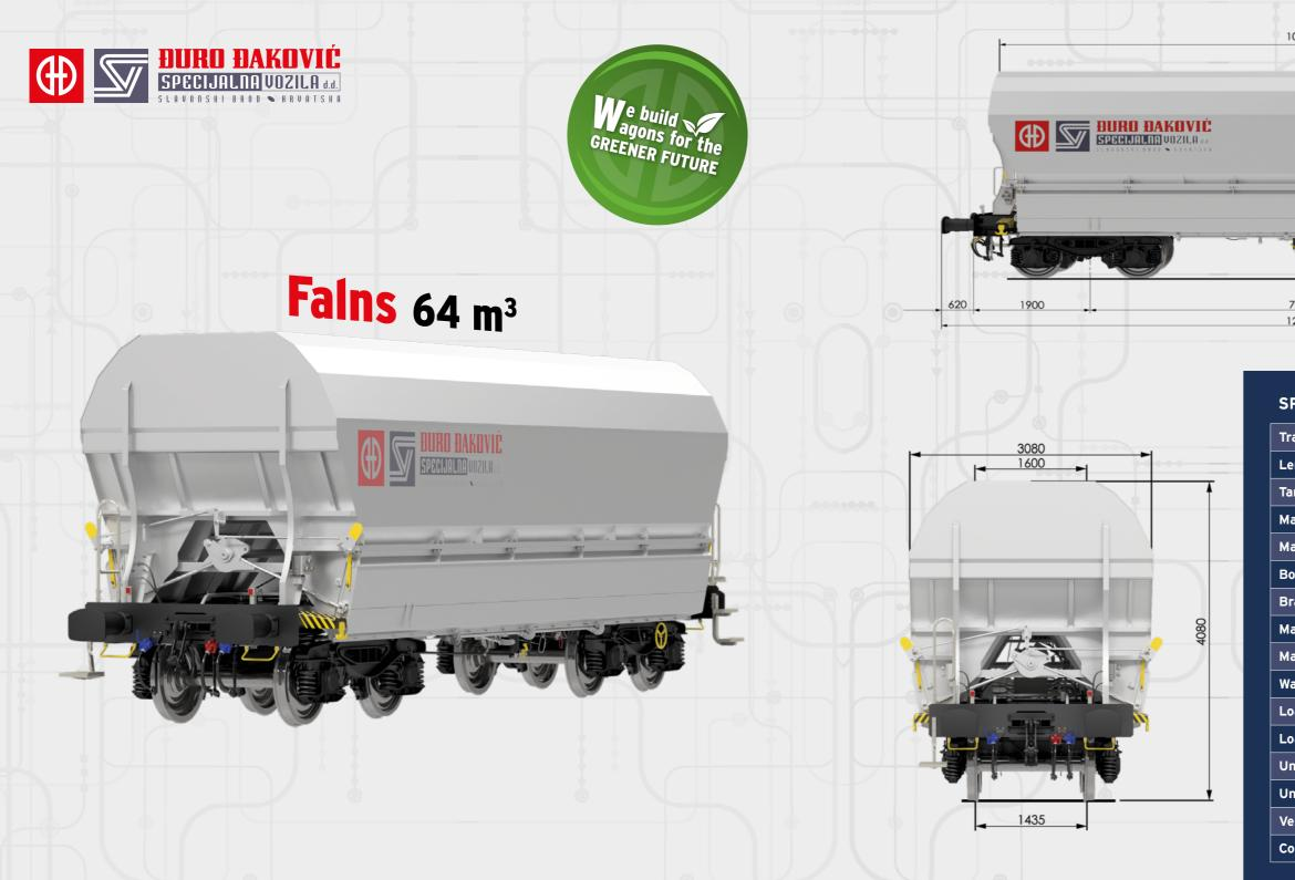
**Fains 64 m**<sup>3</sup> hopper cargo wagon is specifically designed for the efficient transport of limestone and different types of bulk goods which are resistant to weather conditions. Its moderate loading volume and durable construction, combined with large loading opening and one door on each side, providing easy loading/unloading with excellent sealing, makes it perfect for various types of bulk cargo.
