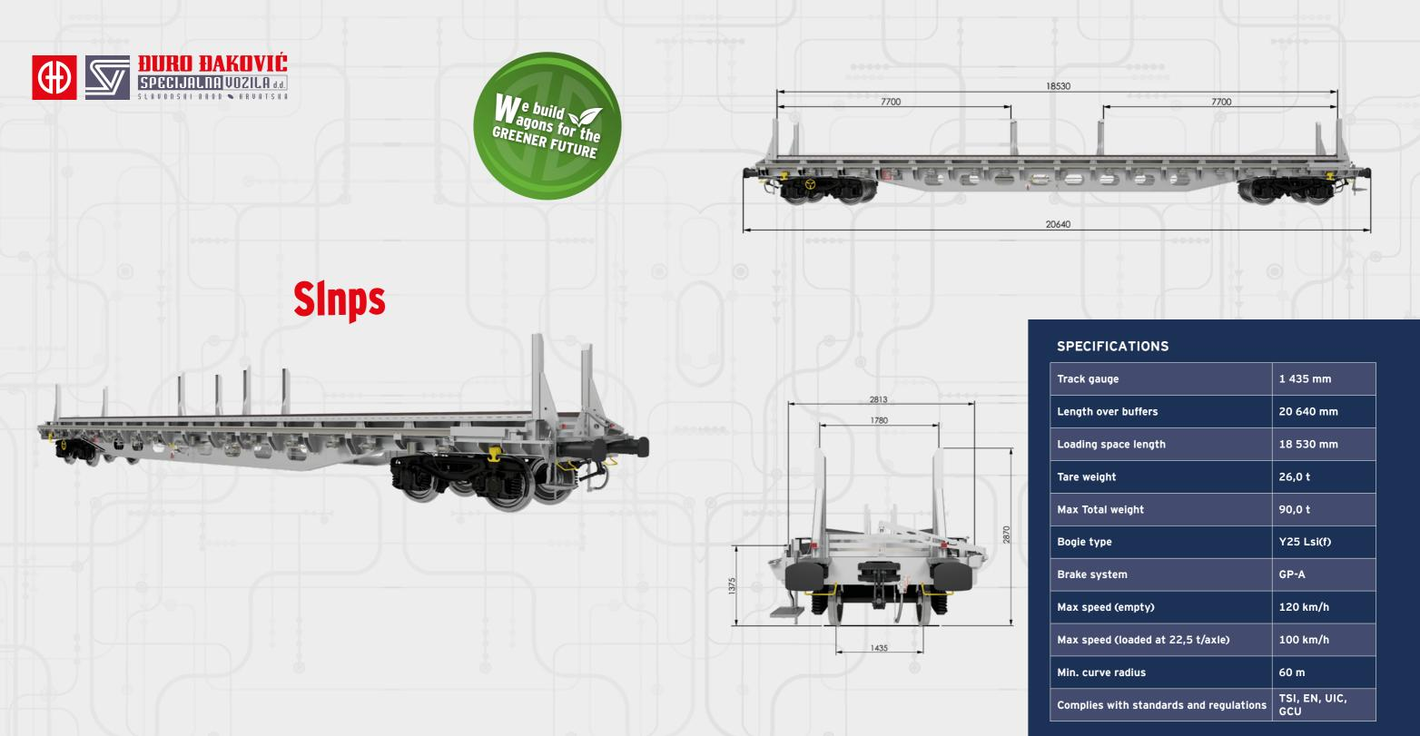
SInps is a specialized cargo wagon designed for transporting different types of railway sleepers during railroad maintenance. The sleepers are loaded and unloaded by a specific gantry crane.
