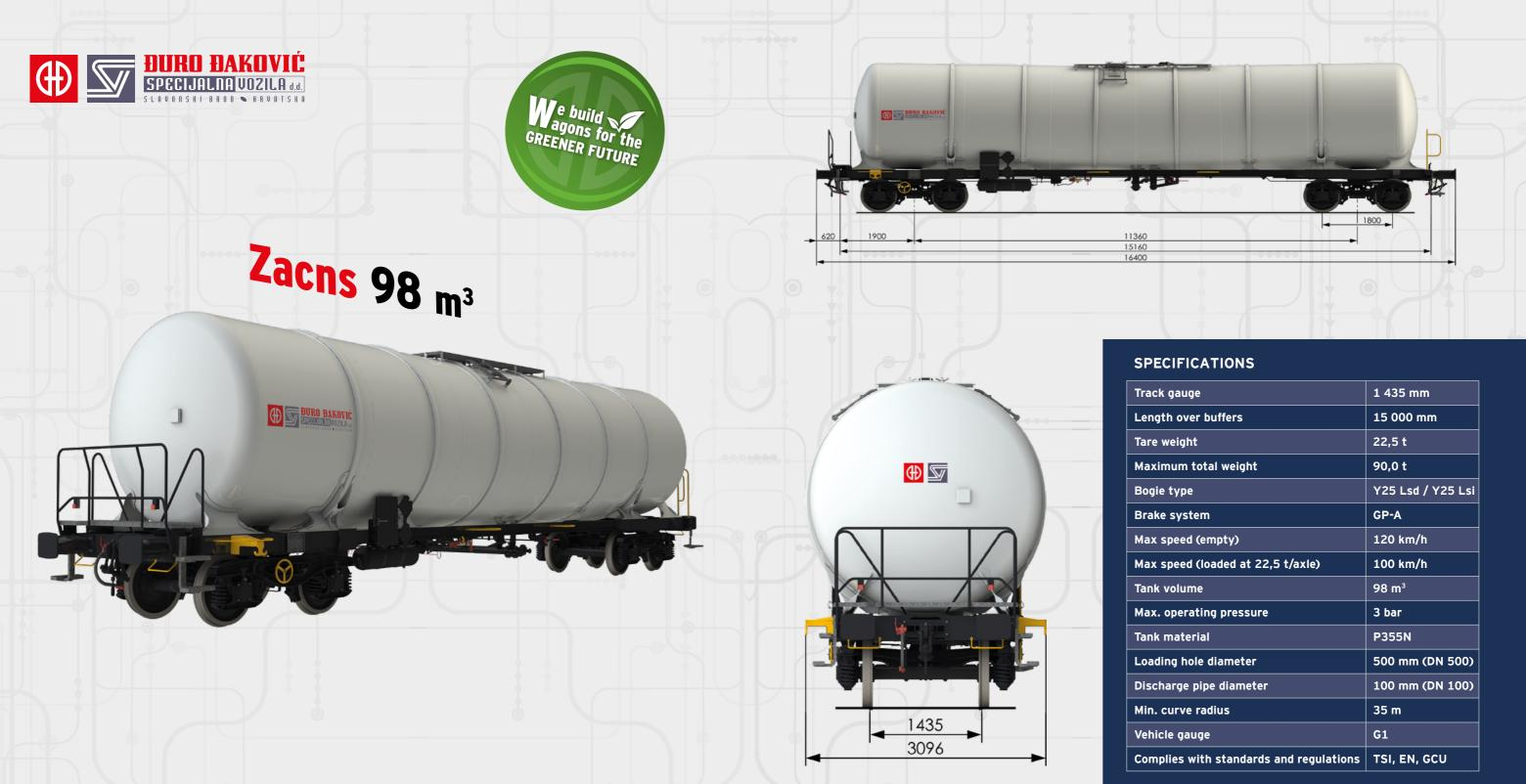
Zacns 98 m<sup>3</sup> is a specialized cargo wagon designed for the transportation of liquid goods, including hazardous substances, it is especially efficient for light density petroleum products. The tank is discharged through the lower side, through the discharge pipe DN 100. The wagon design meets the requirements of RID, TSI, EN, standards and has TEN GE marking for traffic operation.
