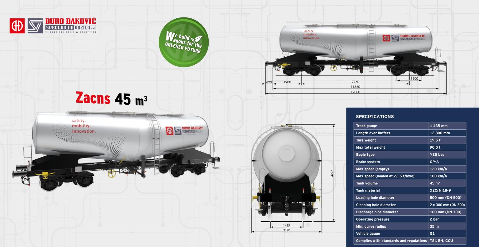
Zacns 45 m<sup>3</sup> is a specialized cargo wagon designed for transporting liquid substances, it is especially effective for carrying CaCo<sub>3</sub> slurry.
