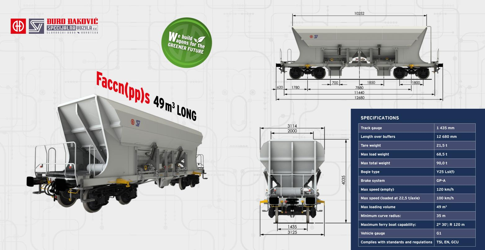
**Faccn(pp)s 49 m<sup>3</sup>** is a specialized cargo wagon designed for transportation of bulk materials not requiring weather protection.
