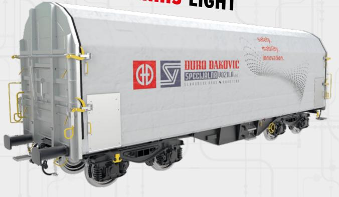
**Shimmns light** is a specialized railway freight wagon designed primarily for transportation of cold steel coils, by placing them in their cradles. Shimmns wagons are a key link in the logistics chain for industries that use large volumes of steel coils, providing a safe, reliable and efficient means of transportation.
