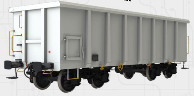
**Eamnos 60 m³** cargo wagon is a versatile and robust open-top freight car. It is specifically engineered to transport heavy, loose, and bulk materials. Its high-sided and reinforced construction makes it ideal for industrial applications, such as scrap metal transport, construction debris removal, and for carrying minerals.
