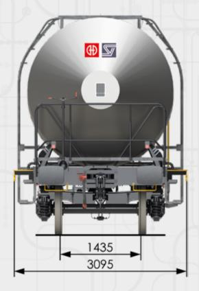
**Zacens 40 m³** is a specialized type of cargo wagon designed for transporting temperature-sensitive liquids, such as certain chemicals, oils, and petroleum products. The presence of a heating system makes them particularly suitable for substances that solidify or become highly viscous at lower temperatures.
