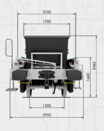
SImnps is a specialized type of cargo wagon designed for railroad infrastructure newbuild projects and maintenance operations. It features a flatbed design with removable containers equipped with standardized fittings to secure them.
