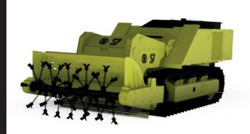
RM-KA-02 is a radio-controlled demining machine designed for mechanical clearing mine contaminated areas by removing all types of vegetation (low, medium-sized and tall plants), treating the soil categories II-V (by splitting, digging and grinding) and destroying all types of antipersonnel and antitank mines (by detonating, splitting and grinding).
