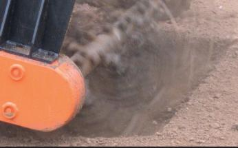
RM-KA-02 is a radio-controlled demining machine designed for mechanical clearing mine contaminated areas by removing all types of vegetation (low, medium-sized and tall plants), treating the soil categories II-V (by splitting, digging and grinding) and destroying all types of antipersonnel and antitank mines (by detonating, splitting and grinding).
